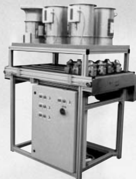
Cooling and drying station for hydraulic pumps
