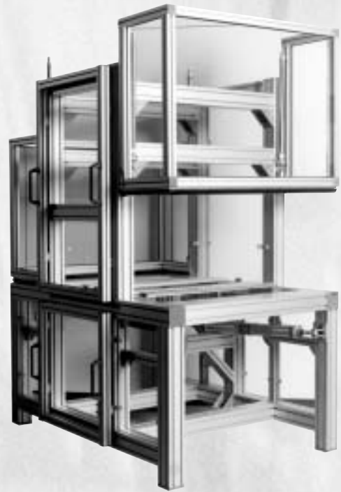
Machine frame with special glass screens for high-temperature application
