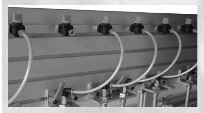
All standard pneumatic elements with thread G 1/8" und G 1/4" can be used with all standard MiniTec profiles. Fixing is possible at any desired point.
